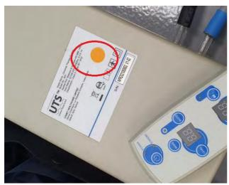
4. plug the power cord into mains outlet. Ensure that electrical cables are safe, tidy, free of obstruction and are not able to be caught in the bed frame. The power LED will be at standby mode with amber light illuminating.
