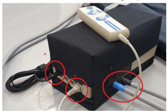
3. Make sure control unit marked with orange dot on product label connects with short ver. of Pad. Control unit without orange dot marked connect with long ver. of Pad.
